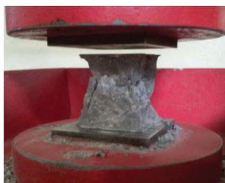
Fig. 4. Compressive strength tests according to EN 196-1:2005 [15]
