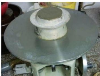
Fig. 2. Consistency tests according to EN 1015-3:1999 [16]
