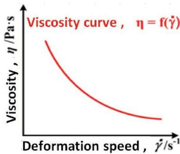
Fig. 2. Typical viscosity curve of pseudo-plastic materials
