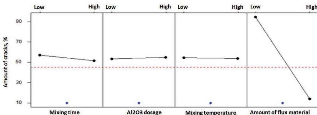
Fig. 9. Susceptibility to cracking, depending on the input mixing parameters
