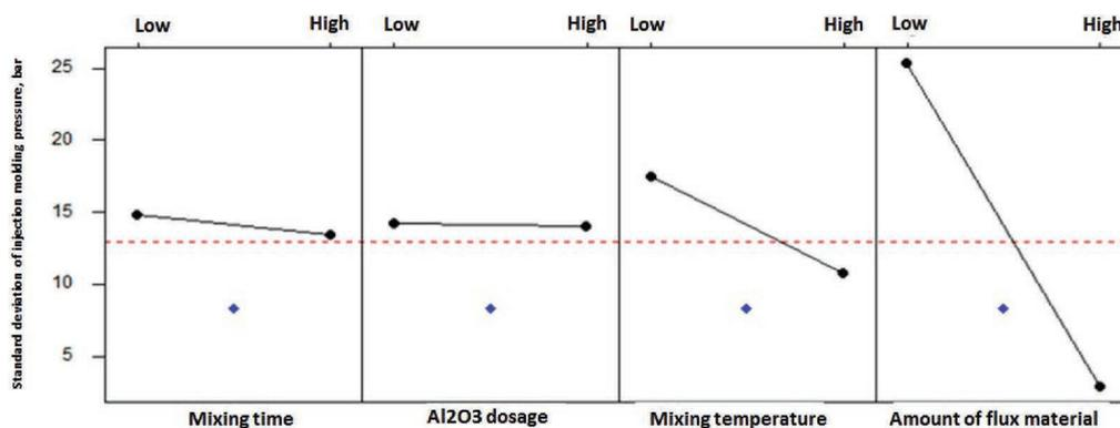
Fig. 8. Influences of input parameters on the standard deviation of injection molding pressure
