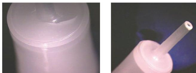
Fig. 1. Cracked (left) and intact (right) sintered alumina ceramic
