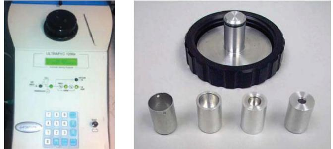
Fig. 3. Quantachrome 1200e type densitometer (left) and measuring cells (right)
