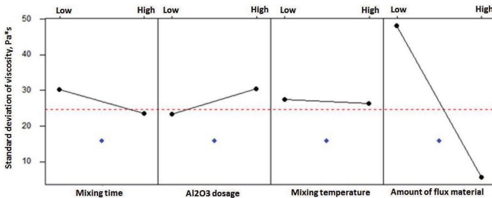
Fig. 6. Influences of input parameters on the standard deviation of viscosity
