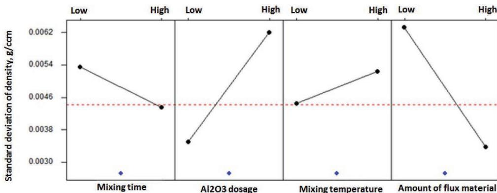
Fig. 7. Influences of input parameters on the standard deviation of density
