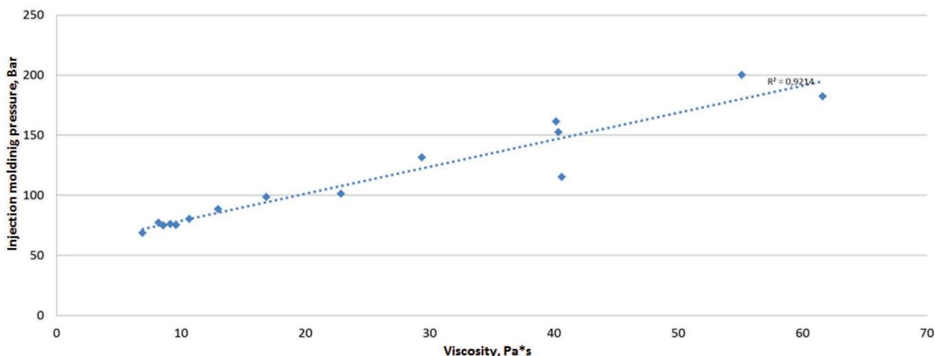
Fig. 4. The determined relationship between the capillary viscosity and injection molding pressure
